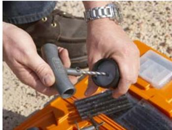
2. Apply lubricant to the spiral shaft of the reamer tool. This will help to probe the hole and temporarily separate the steel belts without damage.
