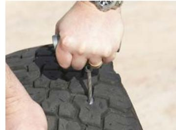
3. Insert the reamer into the puncture hole and push in whilst rotating the handle to clean out the hole. Reinflate tyre to help with insertion of cord.
