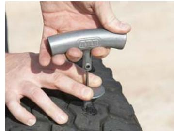
6. To remove the tool, hold the sleeve firmly against the tyre and pull up on the handle. Note: do not twist the handle. Trim the excess protruding cord with a suitable blade.
