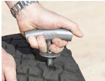
5. Firmly push the insertion tool and cord into the tyre until the sleeve is fully home against the tyre. A small amount of the cord should still be visible.
