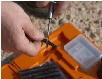
4. Thread the repair cord through the eye of the insertion tool until equal parts are either side of the tool. Lubricant may be added to the tip to make insertion easier.
