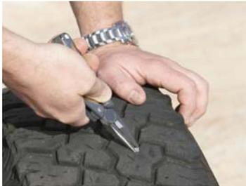
1. Remove debris from tyre tread or sidewall using a suitable tool such as a pair of pliers. Take care, as residual air will escape under pressure.
