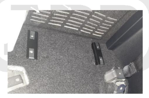
Carefully cut the carpet and fit around the brackets as shown in the above image.
