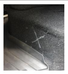
Mark a "X" between the 4x drilled mount holes and carefully cut with a Stanley knife. Behind the carpet is a large hole, where the wiring and air line can be fed from the compressor under the carpet, inside the seat base and then out through the hole as shown.
