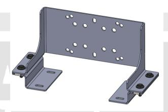
Loosely mount the feet to the compressor bracket using M6x20 bolts & M6 flat washers as shown. Please note the orientation of the feet.
