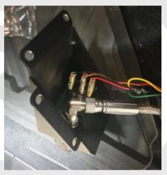
Feed the compressor wiring and air line through the cut carpet and connect to the switch and air coupling. The air line will need a 0740104 90deg elbow.
