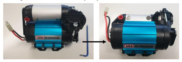
Loosen the bolt holding the manifold using a 10mm spanner. Rotate the manifold 90° as shown. Tighten the bolt to 9Nm [7 lbf.ft].
