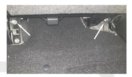
Lift up the rear seat and undo the 5x bolts holding the seat in using a 12mm socket and ratchet.
