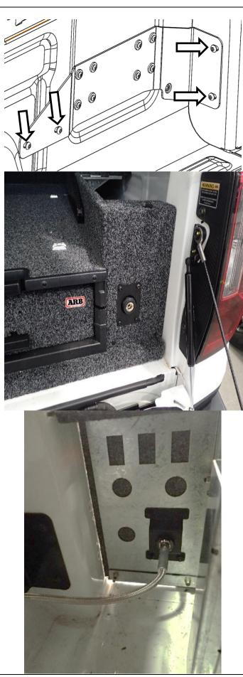
33. Fit four M8 Button head fasteners and tighten to spec.
