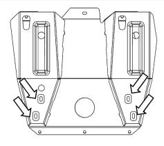
8. Secure the SUMP PANEL to chassis using 4 x M8 bolts and flat washers. **Leave finger tight.**
