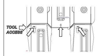
Secure rear of FRONT PANEL to front of SUMP PANEL using 3 x M8 bolts, flat washer and flange nuts. Leave finger tight.
