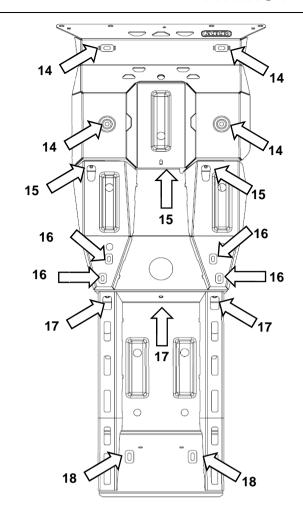
13. Tighten 4 x M8 bolts fixing FRONT PANEL to chassis to prescribed torque.
