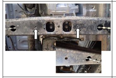
10. Insert 2 x NUT PLATES into transmission cross member and align with holes as shown.
