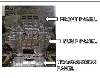
1. <u>ALL VEHICLES</u>: Remove OEM panels from vehicle and retain bolts and fasteners.
