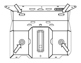
5. Secure the FRONT PANEL using 4 x M8 bolts and flat washers. **Leave finger tight.**
