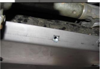
8. <u>ALL VEHICLES:</u> Place 3 M8 cage nuts in rear face of front panel.
