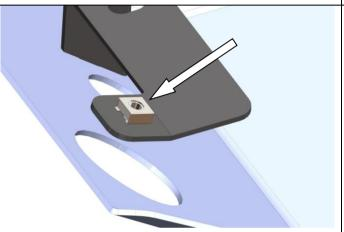
2. **PRADO 150 WITH KINETIC**. Fit two M6 cage nuts to front mounting bracket of panel as shown.
