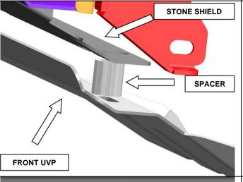
6. <u>120 PRADO</u>. As per image place spacer tube between stone shield and UVP. Secure using M8 x 70mm socket head cap screws, spring washers and flat washers. Leave finger tight.
