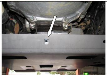
11. Place one M8 cage nut in middle hole of centre panel.
