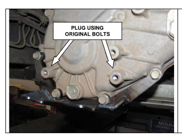
16. Remove original transfer case shield and retain bolts. Remove four lower case bolts and retain. Fit transfer panel as shown using original bolts. Fit remaining bolts into original mount positions at rear.
