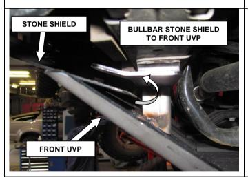
3. Lift front panel into position while placing (if fitted) the bullbar stone shield between the panel and front mounting bracket. Secure panel to chassis using original fasteners and stone shield with M6 bolts removed in step 1. Leave all fasteners finger tight.
