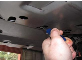
Secure front of centre panel to rear of front panel using three M8 x 25mm bolts, spring washers and flat washers. Leave finger tight.
