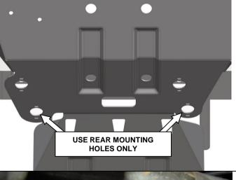
7. <u>120 PRADO</u>. Secure rear of front UVP to chassis using original bolts in the two rear most mounting points only. Leave finger tight.
