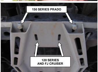
15. **NOTE:** Use outer slots for 150 series and inner slots for 120 and FJ. Secure rear of panel to bracket using two M8 x 25mm bolts, spring washers, flat washers and M8 flange nuts. Tighten all panel bolts when done including front stone shield bolts.
