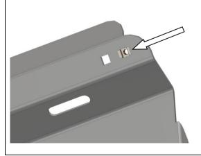
4. **FJ CRUISER**. Fit two M6 cage nuts into front panel as shown. **NOTE:** There are two types of stone shields. Measure distance between O.E stone shield and place cage nuts in correct holes.
