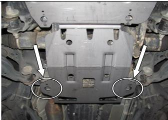
9. Place centre panel on vehicle as shown and secure rear outer mounts to chassis using original fasteners. Leave finger tight.
