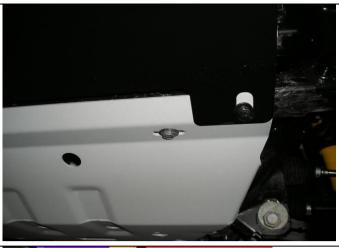
5. Place panel onto chassis making sure it sits under the bulbar stone shield as shown. Secure to vehicle using original hardware removed earlier leaving all bolts finger tight. Secure stone tray to UVP using M6 bolts removed in step 1.
