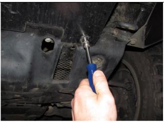
ALL VEHICLES: Remove O.E panels from vehicle and retain bolts. If fitted with a bullbar remove and retain two lower M6 bolts (M8 for Prado 120) and loosen off the top four M6 bolts on the bullbar stone shield.
