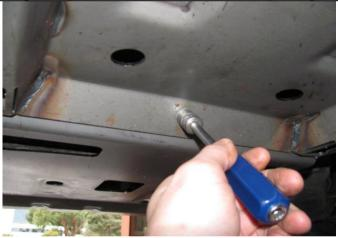
14. Lift transmission panel into place and secure to centre panel using three M8 x 25mm bolts, spring washers, flat washers and flange nuts (outer holes only). Leave finger tight.
