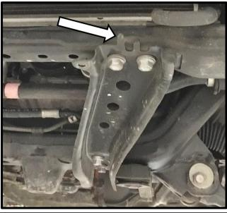
2. Hammer the front right protection panel hook up and out of the way as shown.
