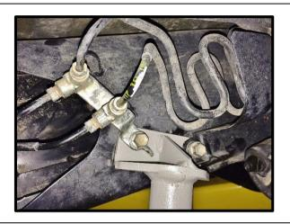
11. Place the fuel line bracket over the 4th panel support plate as shown. Replace the fuel line shroud if equipped. For all holes with factory weld nuts in the frame, fasten with supplied M8 x 25mm hex bolts, spring washer, and flat washer sets. For the holes without factory weld nuts, use a M8 serrated flange nut to secure. Do not tighten these fasteners at this step.
