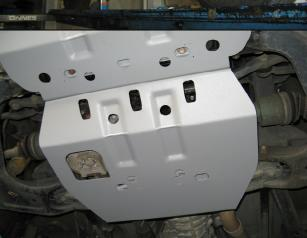
4. Lift sump panel assembly into place and attach to cross member using original M10 bolts. Secure to front panel using 3 x M8 x 35 bolts, spring washers and flat washers. Leave all bolts finger tight. Once this is done insert 1 x M8 cage nut at the centre position at rear of panel.
