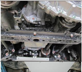
5. Fit mounting plate as shown using original bolts.
