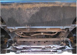
1. Remove O.E stone shields and retain ALL mounting bolts for later use.
