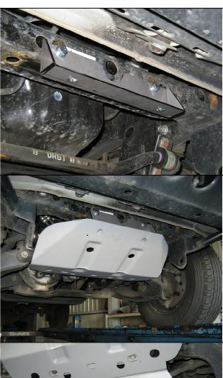
2. Fit front mounting bracket to cross-member using M8 x 35 bolts, spring washers and flat washers. Fit 2 x M8 cage nuts in square holes on top surface of mount. When fitting transmission lines be sure they clear any sharp edges.
