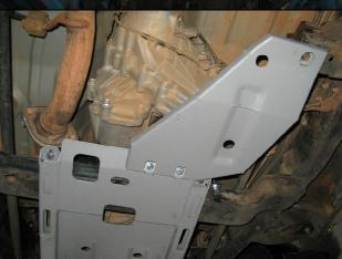
7. Fit transfer case panel using original M10 bolt with large washer removed in vehicle torsion bar mount and 2 x M8 bolts, spring washers, flat washers and flange nuts into transmission panel. Once all this is done tighten all bolts.
