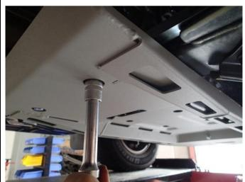
7. Fit transmission UVP and secure to mount bracket using 2 x M10 x 35 bolts, spring washers, flat washers and M10 flange nuts placed on top of bracket. Leave finger tight. Secure to sump UVP using 3 x M8 x 25 bolts, spring washers and flat washers. At this stage tighten all chassis and UVP fasteners as shown by specs below.
