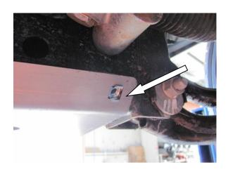
1. Remove original stone shields from vehicle except transfer case. Insert 3 x M8 cage nuts to rear of supplied front panel as shown.
