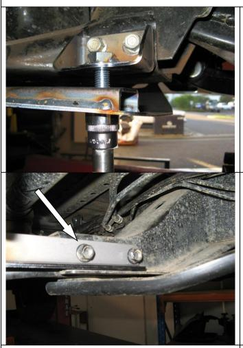
5. Place 3 x M8 cage nuts in rear of sump UVP. Secure sump UVP to chassis brackets using 2 x M12 x 35 bolts, spring washers and flat washers leaving finger tight. Secure front of sump UVP to front UVP using 3 x M8 x 25 bolts, spring washers and flat washers leaving finger tight.
