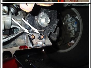
Support front suspension cross member using jack or similar. Remove outer two bolts and fit sump UVP brackets to rear face as shown. Do one side at a time. Leave bolts finger tight.
