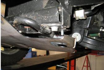
3. Fit front panel as shown by hanging on bolts fitted in step 2. Tighten bolts up slightly to minimise gap but leave loose. Secure rear of front panel to chassis using 2 x M10 x 35 bolts, spring washers and flat washers. Secure front using 3 x M10 x 35 bolts, spring washers and flat washers. Leave fasteners finger tight.
