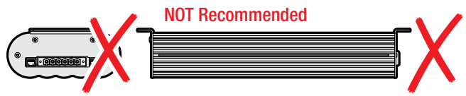
FIGURE 2.2.1.3: Do NOT mount the unit upside down
