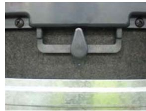
Roller floor locked.
