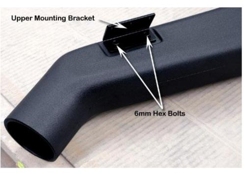
Place a strip of masking tape onto the A-Pillar. Carefully place the snorkel body (Item 1) onto the guard panel. With the snorkel body correctly positioned, mark the upper mounting bracket hole position. (The upper mounting bracket should have approximately 1.0mm gap to the windscreen rubber moulding). Remove the snorkel body from the vehicle and the upper mounting bracket from the snorkel body.
