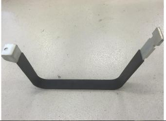
Install the rubber insulation to the inside face of the tank mounting straps.
