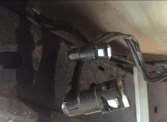
Re insert the white retaining clips into the fuel lines on the vehicle.
