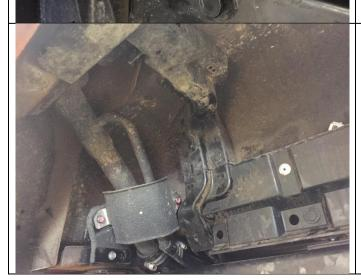
Re-install the small metal shield over the filler neck. Re-install the2 plastic trims over the top of the wiring harness and rollover vent.
