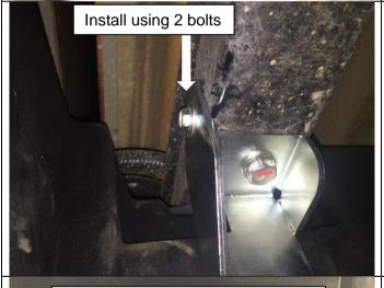
Secure other end of strap with the original bolts retained in the tank removal procedure.
