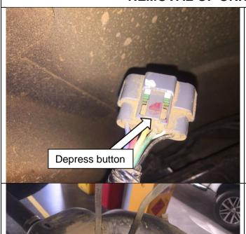
Whilst lowering tank disconnect the sender wiring from the top of the tank.
