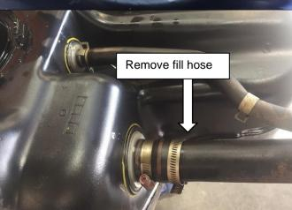
Remove the 35mm fuel filler hose from the fuel tank. Retain hose and clamps.
