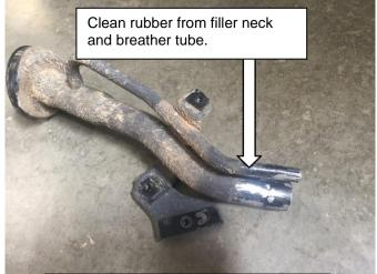
Clean the rubber coating from the outside of the tube so that they can accept hoses when reassembled.
