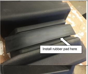
Remove the white paper backing from the 400mm long rubber insulator and install on the front of the tank as shown.
