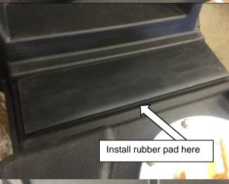
Remove the white paper backing from the 320mm long rubber insulator and install on the rear of the tank as shown.
