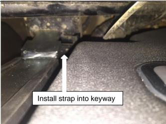
Once the tank is in place insert the new rear mounting strap into the keyway in the chassis.
