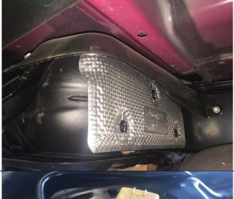
Remove shield from top of cross-member at the front of the fuel tank.
