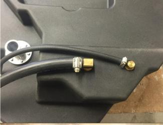
Install the 16mm and ¼ fuel hoses to the filler breather and the rollover valve on top of the new tank. Secure these hoses using the clamps supplied in the kit.
