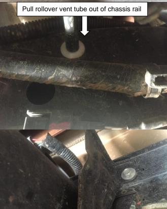
Remove rollover vent tube from the chassis rail by pulling outward. The tube is located on the inside of the chassis rail near the filler neck.
