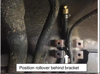
Position the rollover breather hose behind the bracket that mounts the plastic trims in the LHR wheel arch. Secure the hose and install the rollover vent into the hose. Secure the vent with the hose clamp supplied in the kit.
