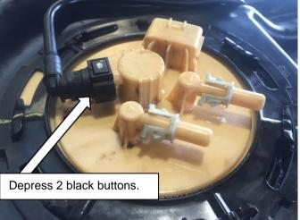
Remove the rollover breather tube from the fuel sender. To remove the tube depress the 2 black buttons and pull.
