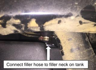
Install original fuel filler hose retained in the removal procedure to the filler neck on the Frontier tank. Secure using the hose clamp retained in the removal procedure.
